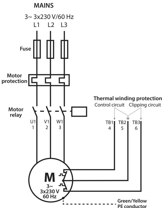
Connection of the thermal winding cover
